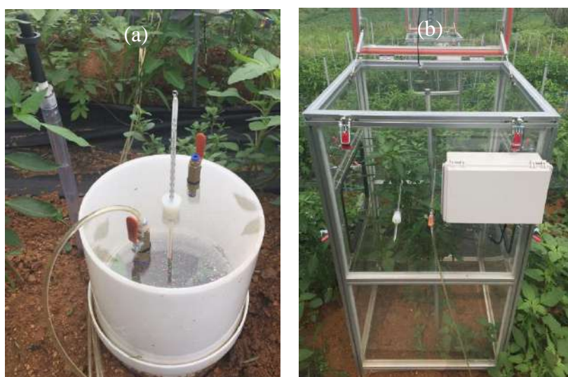
Fig. 1. Dynamic flow-through chamber methods for ammonia gas trapping (a: soil ammonia emission without plant; b: canopy ammonia flux with plant)
